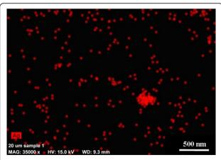
**Figure 4 SEM-EDS mapping of nanosilver aerosols deposited on TEM grid during the exposure**. The colored dots represent the elemental map for Ag at the expected characteristic X-ray energy for Ag and show, based on size, the presence of silver nanoparticle agglomerates.
